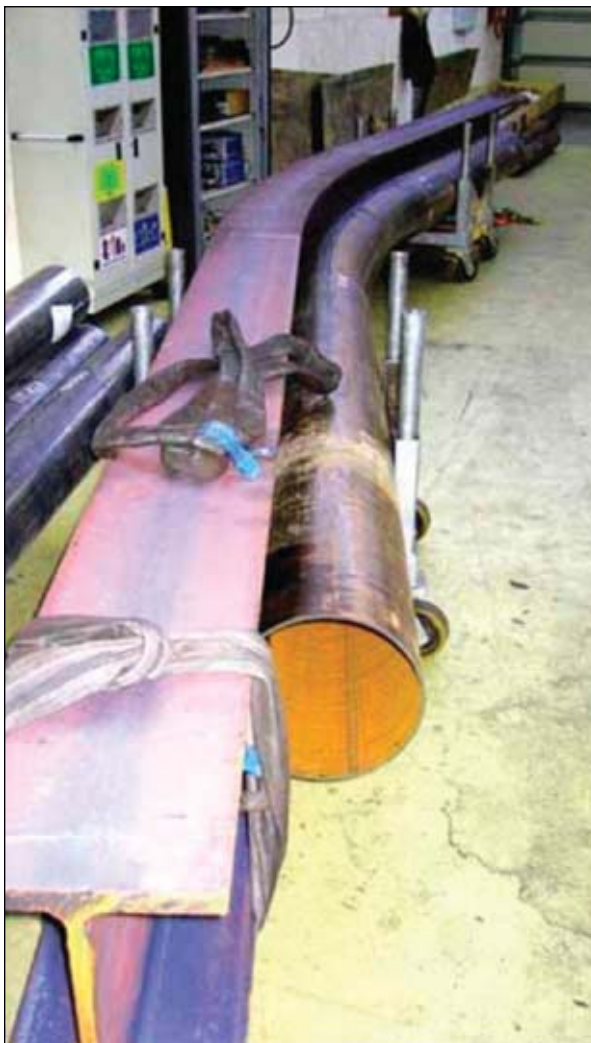
Testing has shown that SET technology can successfully be used in pipeline contexts through bends up to 20° (Fig. 7).
